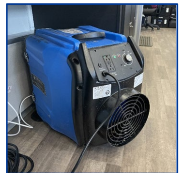
An Air Scrubber is a fan with a multi-layer particle filter system housed in a ruggedized case.
